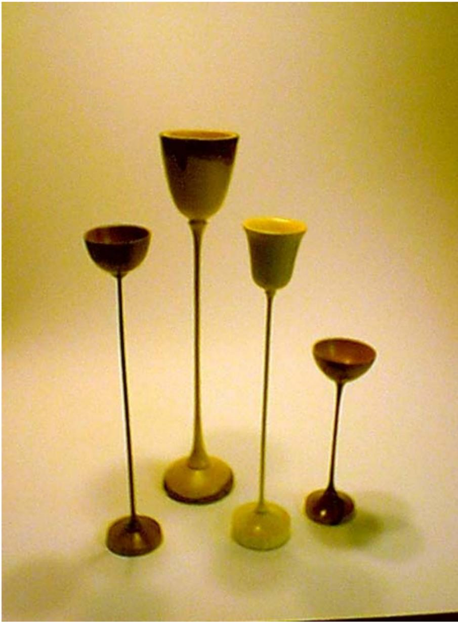
Chucking: Use spigot or 3 jaw type chucks. Try to use the full back to front depth for better holding power. The long overhang from the headstock makes this attribute very critical to the project. Shallow jawed Nova/Oneway chucks have holding limits. A tenon cut on the blank aids with holding. Accept the fact that some of the wood length must be dedicated to holding the work.
