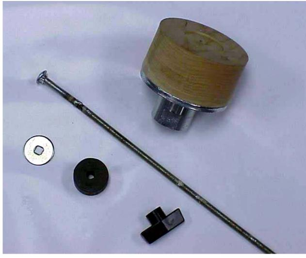
I have a hand-wheel on my lathe, and the center is tapered slightly. I turned a wooden plug to fit that taper, and extend out about a ½". The threaded rod should be just long enough to pass through this plug by about a ½ to ¾" when the compression plug is "uncompressed". The faceplate and plug are center bored for the diameter of the threaded rod, centering the compression plug when in use. A threaded knob is threaded
