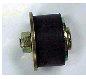
I have begun using a different method for jam chucking which allows me to avoid having to turn a jam plate for each individual piece. This method uses a rubber compression fitting - commonly available at the hardware store in either automotive or plumbing departments. These plugs come in various sizes and as they are compressed in thickness, they expand in diameter, creating a snug fit.
