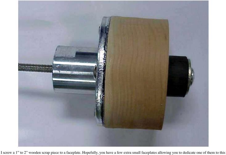
function. Turn the piece round and square off the face. Next, taking the bolt from the compression fitting. I had a piece of threaded rod welded onto the end. I made it long enough to easily pass through the wooden faceplate, metal faceplate, and the headstock, leaving a couple inches out the outboard end.
